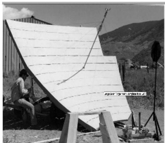
Fig. 9. Experimental solar furnace with parabolic mirror [10]
