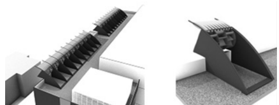
Fig. 2.6.2. String of cornice modules I Installed on building roof
