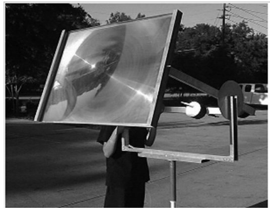
Fig. 8. Experimental solar furnace with Fresnel lense [10]
